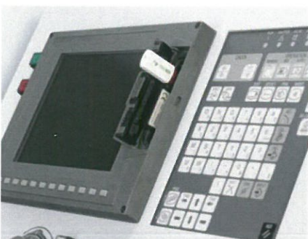
NC program I/O NC programs can be input and output using a USB memory stick or compact flash card.
