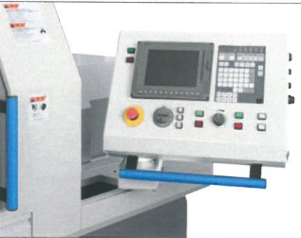
Position adjustable operation panel By swiveling the position adjustable operation panel, you can perform operations while viewing the machining area.
