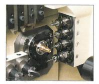
●4-Spindle Endworking / Backworking Attachment For customers who need to perform more versatile machining
